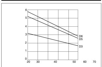
Derating curve is used for finding max. load current at an elevated ambient temperature. The 3 lines in the graph represent the 3 nominal current ratings of the RP1 series (RP1...D3/D5/D6).
