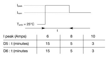
Note: Even though the D3 can withstand a slight increase in current for a limited time, it is not recommended for this purpose.
