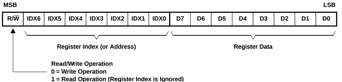
Figure 24. Control Data Word Format for MDI
