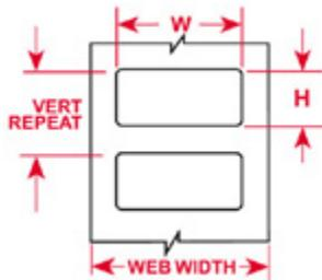
Printable, polypropylene labels for thermal transfer printers. Please Note: This material is UL & CSA approved with its respective ribbon. See the "Recommended Ribbon Series" for the appropriate ribbon to use.
