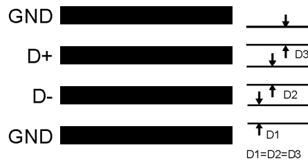
Figure 12. Ideal Diode Trace Layout
