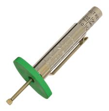
PCL's "Made in Sheffield" Tyre Tread Depth Gauge is manufactured to stringent quality standards and is VOSA approved for MoT testing.
