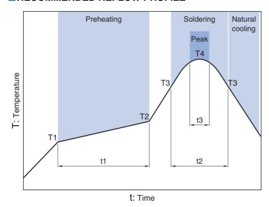
Preheating Soldering Peak Temp. Time Time Temp. Temp. Time T1 T2 T4 Т3 t3 150°C 180°C 90 to 120s 230°C 40s 245°C 5s max.
