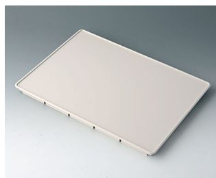
B4146107 Front panel L ABS (UL 94 HB) off-white RAL 9002 10.85"x7.70"x0.61"
