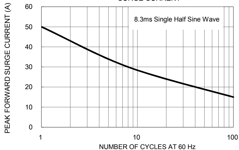
FIG. 3- MAXIMUM NON-REPETITIVE PEAK FORWARD SURGE CURRENT
