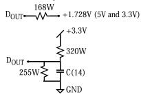
Figure C: 3.3V Output load
