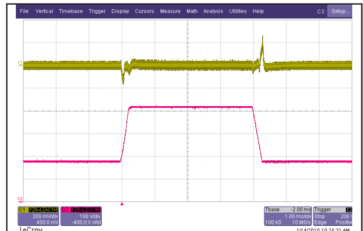
Figure 6: Output voltage response to step-change in input voltage (180V - 425V - 180V), at 50A load current. Load cap: 15μF tantalum capacitor and 1μF ceramic cap. Ch 1: V out (200mV/div), Ch 2: V in (100V/div).
