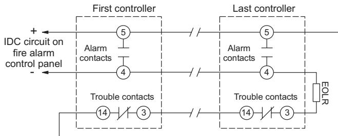
End-of-line resistor required on last device for circuit supervision.
