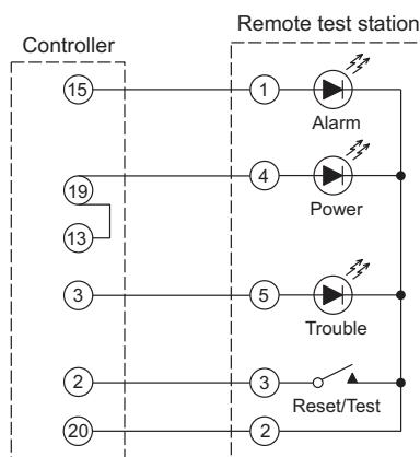
**Note:** For applications where only the Alarm LED and Reset/Test switch is required, wiring the Power LED and Trouble LED is optional.
