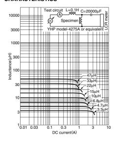
Test equipment L: 4194A IMPEDANCE/GAIN-PHASE ANALYZER HP, or equivalent (Measured at 100kHz/0.5V)
