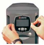
2. Rotate the mimic panel counter clockwise and then secure it back in place
