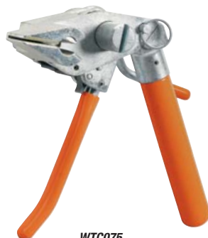
WTC075 Designed to install ¼" to ⅝" wide Free-End Clamps. The lightweight, ratchet-action tool tension cuts and secures the buckle tab.
