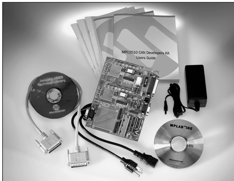
Figure 2.1: MCP2510 Development Kit Components
