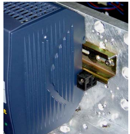
Fig. 23 One of 4 DIN-rail fixing brackets
