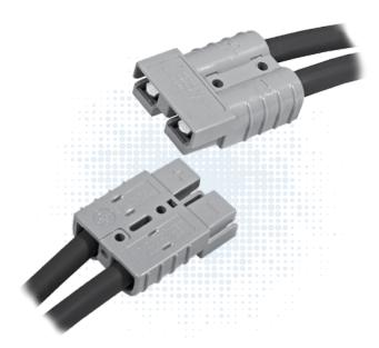
Based off the design pioneered by Anderson in 1953, the two pole SB® connectors set the standard for DC power distribution and battery connections. SB®50 connectors feature a one piece plastic housing using stainless steel springs to hold low resistance contacts in place. Wires sizes from #16 (1.5 mm²) to #6 (13.3 mm²) are held in the smallest of the SB® series housings.
