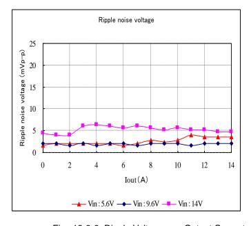
Fig. 12-3-3. Ripple Voltage v. s. Output Current
