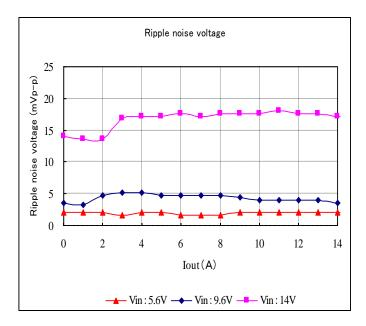
Fig. 12-3-9. Ripple Voltage v.s. Output Current
