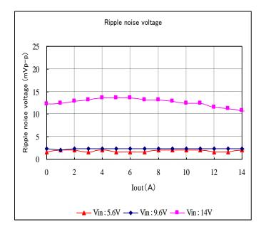
Fig. 12-3-6. Ripple Voltage v.s. Output Current
