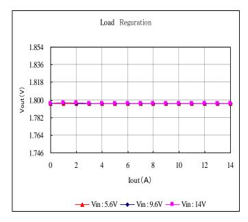
Fig. 12-3-7. Output Voltage v.s. Output Current
