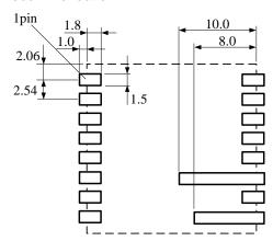
There are wiring coppers or through-hole via at the bottom side of the DC-DC converter. When you design your PCBs, please be careful not to short the circuit of the DC-DC converter or PCBs.
