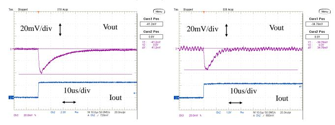
Fig. 12-1a. Load Transient Response (MPDRX301S)
