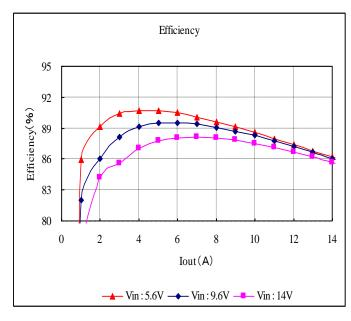
Fig. 12-3-8. Efficiency v.s. Output Current
