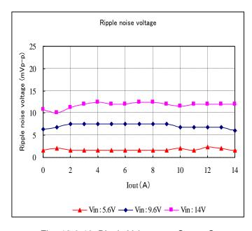
Fig. 12-3-18. Ripple Voltage v.s. Output Current
