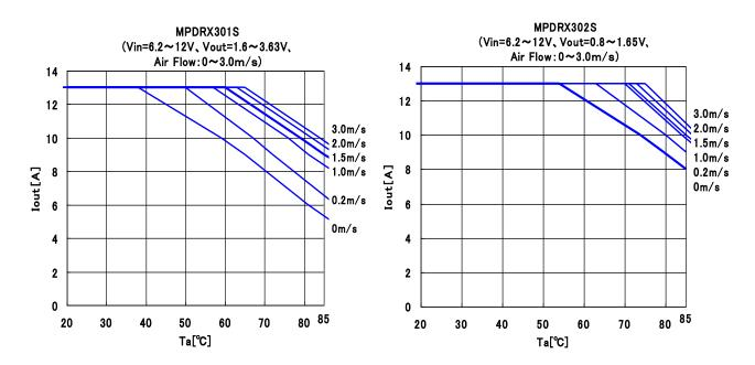
The above derating limits apply to this product soldered directly to 101.6\*180mm\*1.6mm PCB (6 layer). Any adjacent parts of high temperature may cause overheating. For reliable operation, please ensure that the FET temperature of this product is maintained below 120°C and the inductor temperature is below 111°C.
