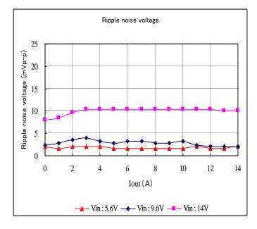
Fig. 12-3-15. Ripple Voltage v.s. Output Current
