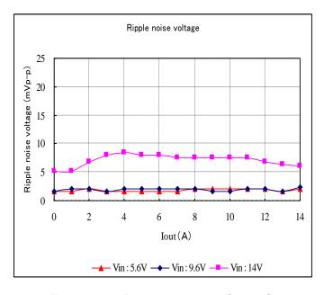
Fig. 12-3-12. Ripple Voltage v.s. Output Current
