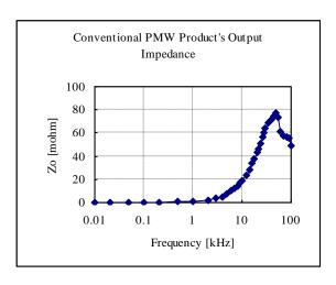
Fig. 12-2-1. Output Impedance of MPDRX301S/302S
