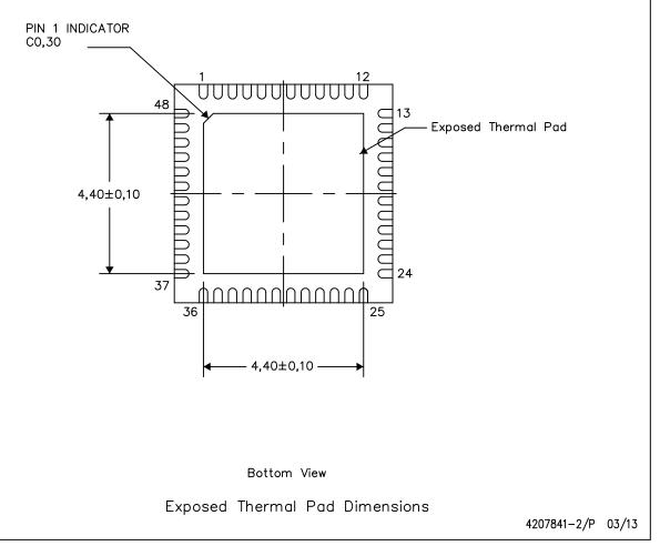
NOTE: All linear dimensions are in millimeters
