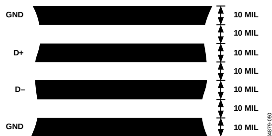
Figure 50. Arrangement of Signal Tracks
