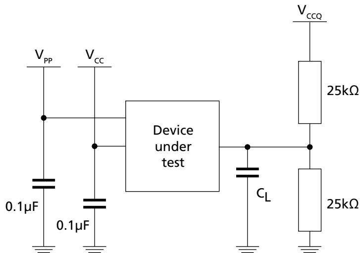
Note: 1.  $C_L$  includes jig capacitance.
