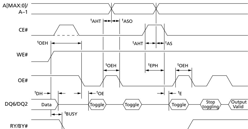
Notes: 1. DQ6 stops toggling when the PROGRAM or ERASE command has completed. DQ2 stops toggling when the CHIP ERASE or BLOCK ERASE command has completed.
