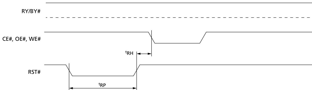
**Figure 15: Reset AC Timing During PROGRAM/ERASE Operation**
