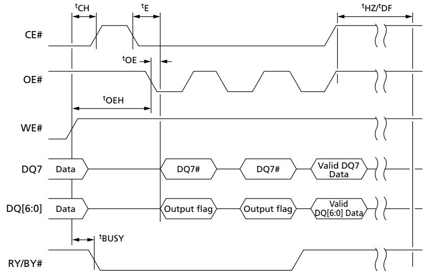
Notes: 1. DQ7 returns a valid data bit when the PROGRAM or ERASE command has completed.
