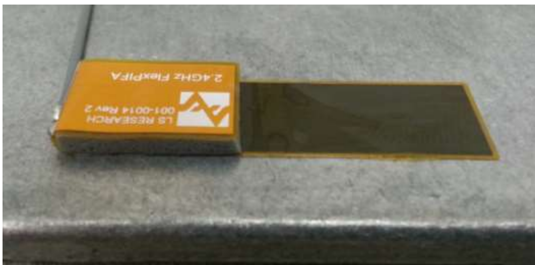
Figure 27 FlexPIFA Mounted on Metal
