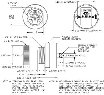
NOTE B: MOUNTING- REMOVE BLACK PLASTIC NUT AND INSERT THREADED FRONT THROUGH 1.25' HOLE PUNCHED IN PANEL, IF DRIENTATION IS NEEDED, NOTE LOCKING FLATS ON DRAWING. SCREW NUT BACK ON. DO NOT OVERTIGHTEN.
