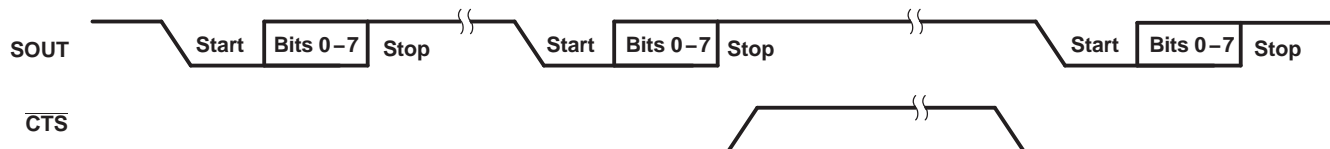
Figure 3. CTS Functional Timing Waveforms
