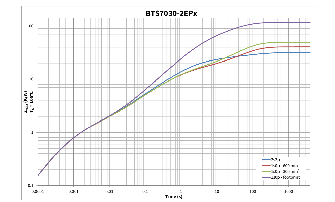
Figure 9 Typical Thermal Impedance. PCB setup according Chapter 4.4.1
