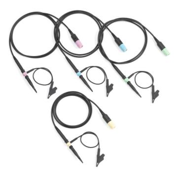
The THP0301 probes are 300 MHz, 10X passive voltage probes with 10  $\text{M}\Omega$  input resistance. These probes are for use with the THS3000 Series oscilloscopes and are color coded to match the oscilloscope's channel input connectors, front-panel channel selector buttons, and the displayed waveforms.
