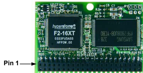
Figure 5: iDiskOnChip Horizontal Version 44 pin, Left-Oriented
