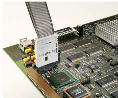
E5346A 34-channel Mictor connector probe
