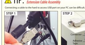
Simply connect the mountable extension cable once to the USB port on the back of your computer
