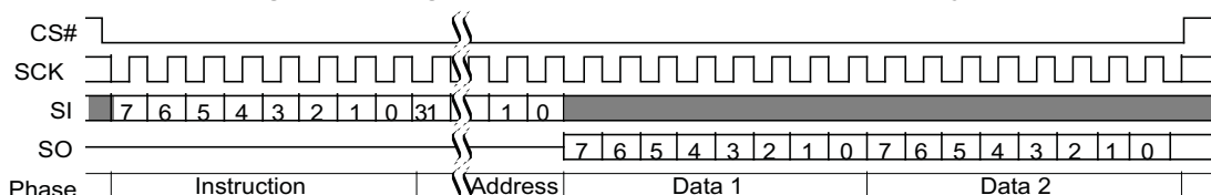
Figure 10. Single Bit Wide I/O Command without Latency
