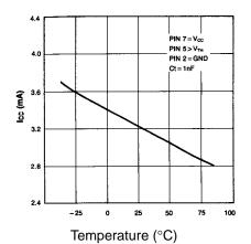
Figure 2. Temperature Drift (IOC)
