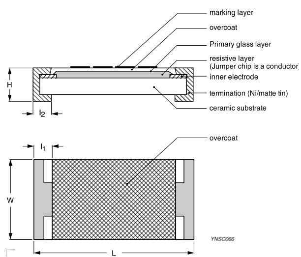
Fig. 5 Chip resistor outlines
