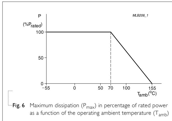
Fig. 6 Maximum dissipation ( $P_{\max}$ ) in percentage of rated power as a function of the operating ambient temperature ( $T_{\text{amb}}$ )
