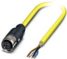
Sensor/actuator cable, 4-position, PVC, yellow, shielded, free cable end, on Socket straight M12 SPEEDCON, cable length: 5 m
