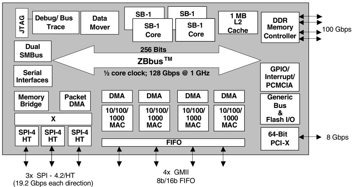
The **BCM1480** device is an MIPS64 processor core-based system-on-a-chip (SOC) that offers industry-leading performance, high functional integration, and low-power levels required by next-generation computing, storage, and networking applications.
