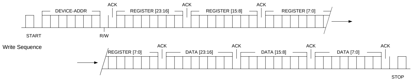
FIGURE 14. I²C WRITE SEQUENCE OPERATION
