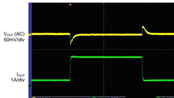
Load Transient Response ( V_{IN}=3.3V , V_{OUT}=2.5V , I_{OUT}=0.5A to 3A )
