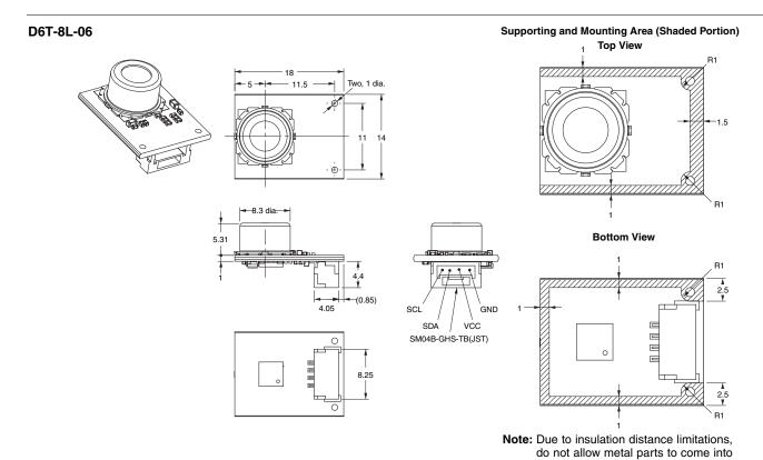
**Note:** Unless otherwise specified, a tolerance of  $\pm 0.3$  mm applies to all dimensions.
