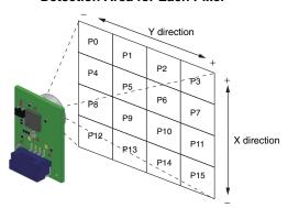
Note: Definition of view angle: Using the maximum Sensor output as a reference, the angular range where the Sensor output is 50% or higher when the angle of the Sensor is changed is defined as the view angle.
