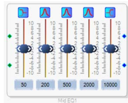
Figure 29. Configured 5-Band EQ Cell
