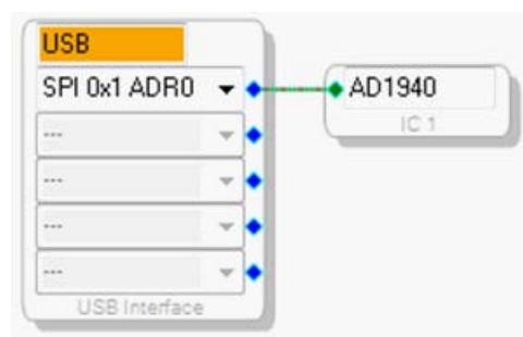
Figure 14. Connecting the USBi to an AD940 IC
