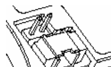
Figure 9: Master Setting for Vertical iDiskOnChip 40-Pin Connector
