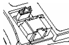
Figure 7: Slave Setting for Vertical iDiskOnChip 40-Pin Connector
