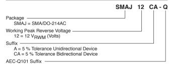
Q = AEC-Q101 Compliant, 13-inch Reel QH = AEC-Q101 Compliant, 7-inch Reel
