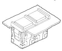
Drawing shows two switches, slot mounted. From left to right: one center barrier, a second switch, plus another end barrier to complete the arrangement.
