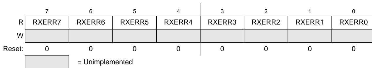
Figure 12-17. MSCAN Receive Error Counter (CANRXERR)
