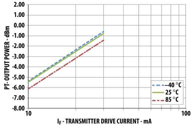
Figure 6. Typical optical output power vs. drive current
