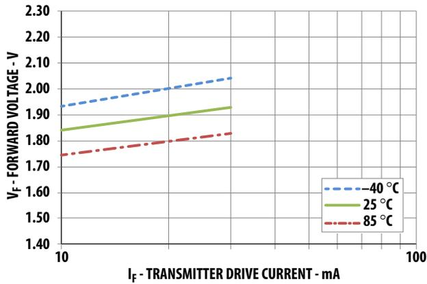
Figure 5. Typical forward voltage vs. drive current
