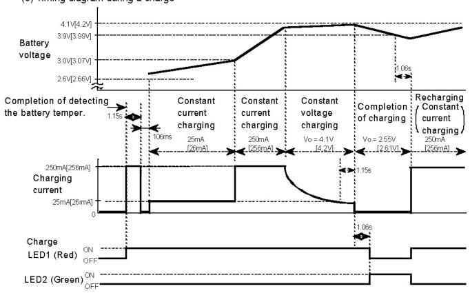
Charge Control IC for Li-Ion Batteries
