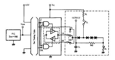
Notes) 1. C<sub>L</sub> includes probe and jig capacitance.
