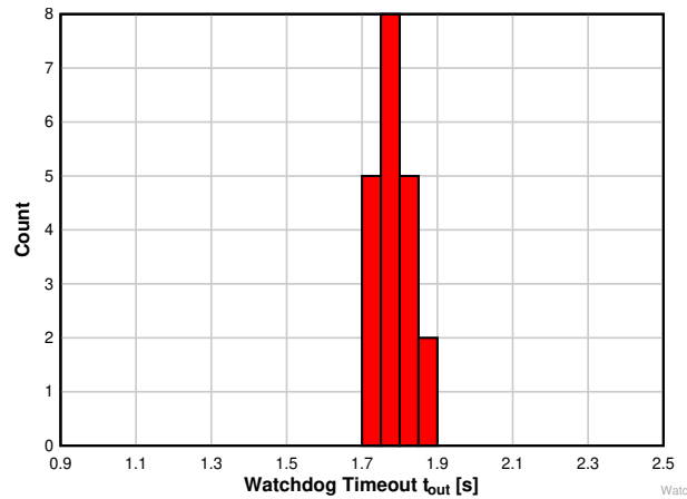
Figure 6-14. Watchdog Timeout Histogram for TPS3823A-33 Devices at 125°C (Unit Count = 20)
