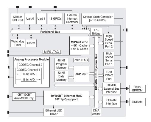
The Broadcom **BCM1115** is designed for use in cost-sensitive, single Ethernet port, Enterprise IP Phone products. The **BCM1115** is complementary to the BCM1101 VoIP CPE engine, which is ideally suited for higher-end, two-port Ethernet VoIP products that require an integrated Ethernet switch and a second Ethernet port.
