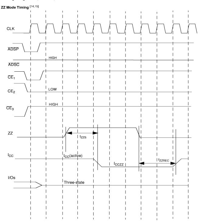
Device must be deselected when entering ZZ mode. See Cycle description for all possible signal conditions to deselect the device.
