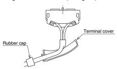
3. If using a VVF wire, bend the wire towards the unit, and once it has taken the proper shape, install the terminal cover. After installing the terminal cover, attach the rubber cap.
