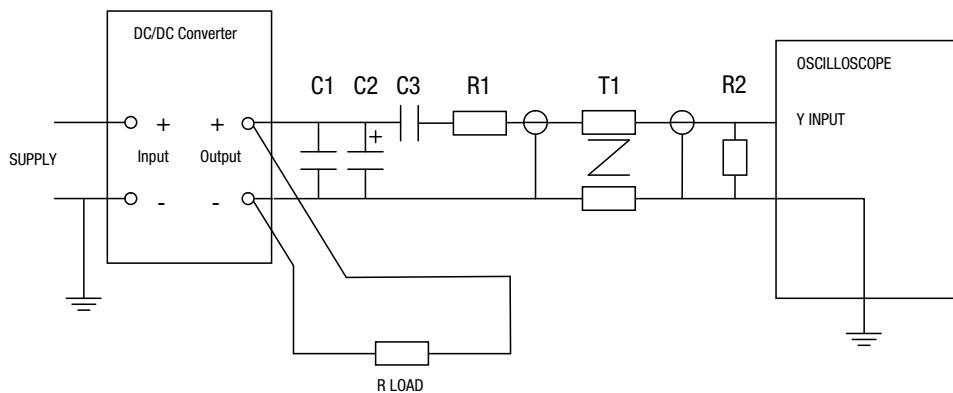
**Input Reflected Ripple Current Test Method**
